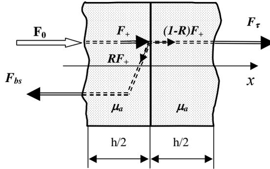
**Fig.4.** One scattering layer of 1D phantom of turbid media.
