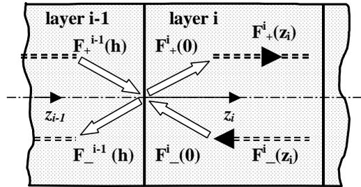
**Fig.3.** Geometry of internal boundary processes.
