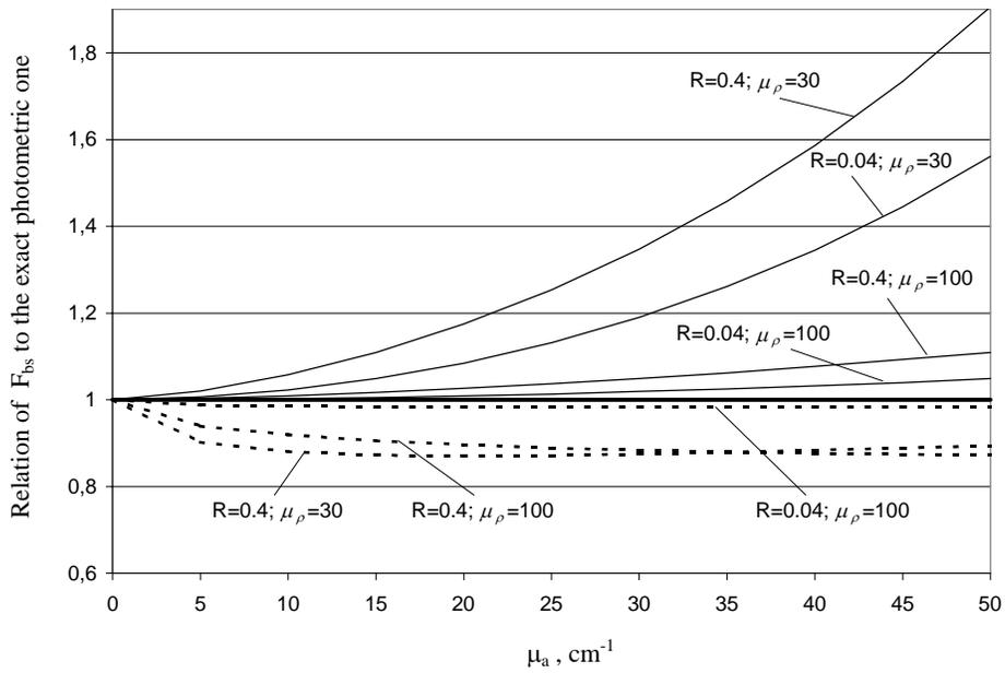
**Fig. 6.** Errors in  $F_{bs}$  with the increase of absorption.
